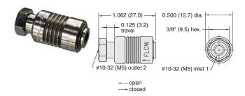
Medium: Air Mounting: In-line or direct to fitting
