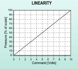
This chart shows the linear characteristics of QB3 products when given a ramp signal from 0-10 volts. Characteristics would be similar for 4-20 mA units.
